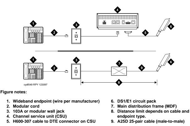
If using a **CSU**, the distance between connections may be up to 1300 ft. (397.2 m). The maximum distance to the endpoint depends on the type of cable and the specifications of the endpoint.
